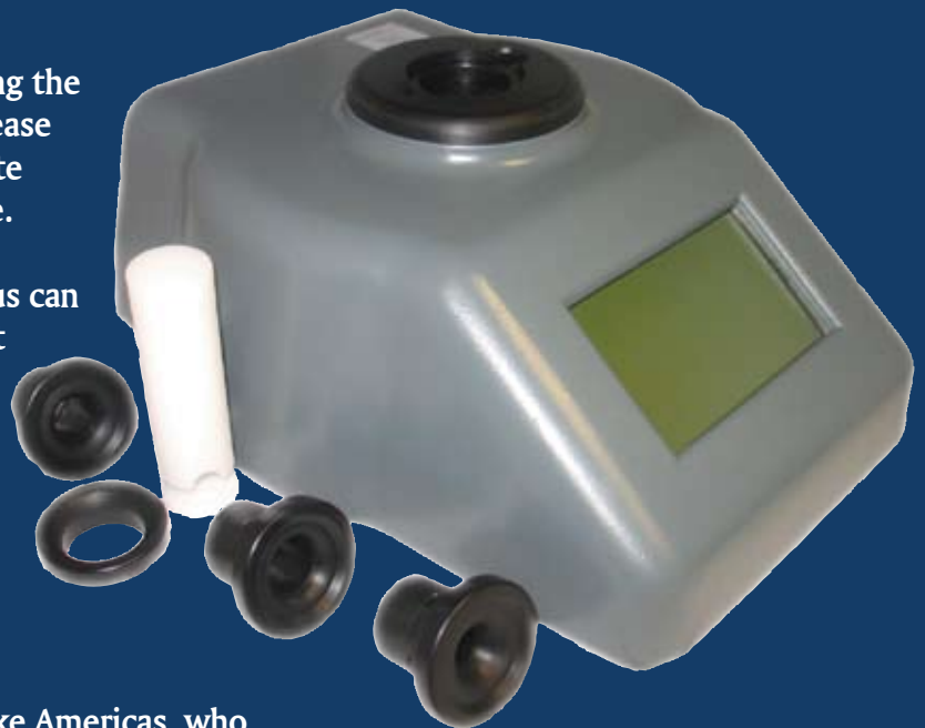
Kittiwake's new ferrous debris monitor, the ANALEX fdMplus
