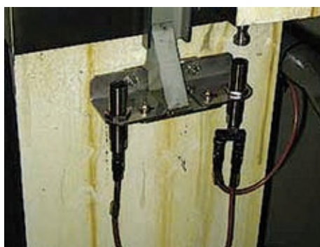
BWMS is designed to monitor bearing wear in 2-stroke engines.
