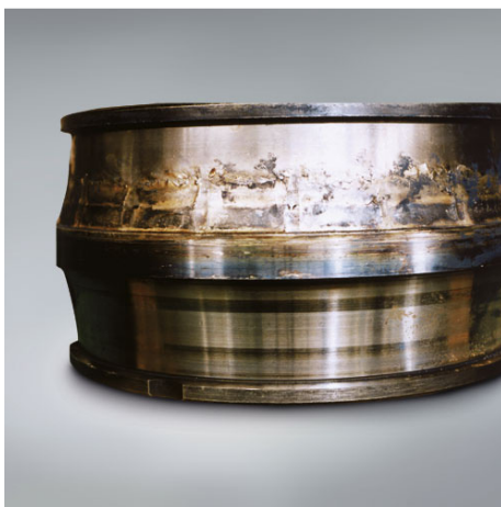
Figure 2: Damaged inner ring of a spherical roller bearing caused by insufficient lubricant.
