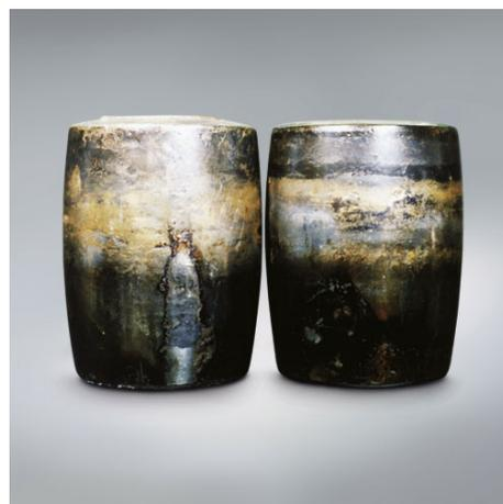
Figure 3: Damaged bearing rollers caused by insufficient lubricant.
