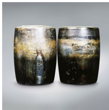
Figure 3: Damaged bearing rollers caused by insufficient lubricant.
